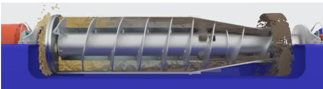
Figure 2. Shallow cone configuration
